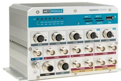
Swindon, Wiltshire – URGROUP (UK), a leading provider of Digital Train Enhancements, is delighted to introduce to the UK rail industry the NB3800 Cellular Router manufactured by Net Module (a Belden company). With dual 5G radios, 4 Sims, 5 Ethernet Ports and GNSS, the NB3800 is one of a range of routers for on-board mobile network data and voice communication for Off-Train Mobile Comms Gateway (MCG) by Net Module.
